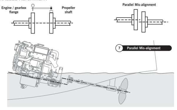
The engine mountings and the couplings must now be tightened in position and the alignment re-checked.
