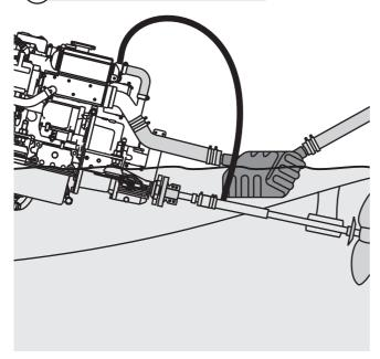
**Beta 10 to Beta 60** - can be connected to the heat exchanger end cap using our 'Stern Bleed kit' and drilling and tapping the end cap.
