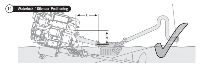
You should always create a 'gooseneck' with the exhaust hose (or purchase a propriety one) by raising the exhaust hose 40 cms above the waterline before exiting the transom at least 5 cms above the waterline. This will stop any waves pushing seawater down the exhaust.
