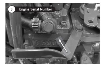
The engine serial number is shown on the rocker cover label. It is also stamped on the crank case flange below the fuel injection pump on the starboard side of the engine.
