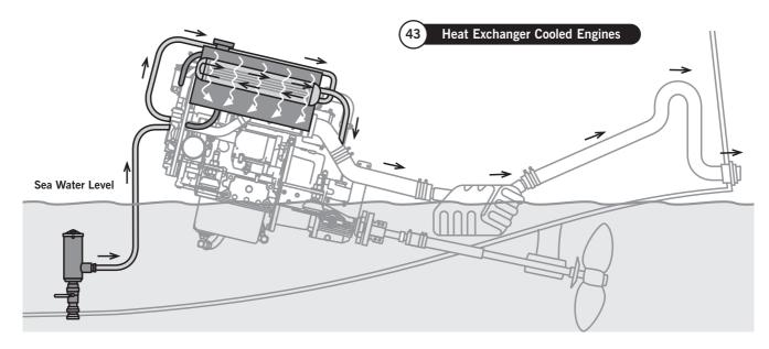
All diesel engines require a cooling system. Generally all modern seagoing boats with wooden or GRP (Glass Reinforced Polyester) hulls normally have a Heat Exchanger 'Fresh Water' cooling system.
