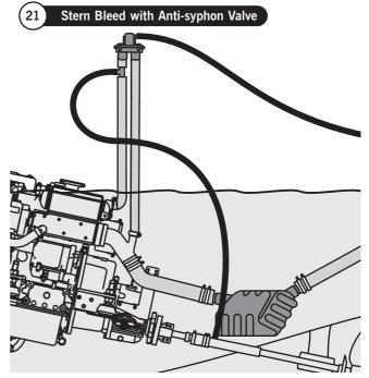
**Beta 75 upwards** - need a 'T' piece with an 1/8" BSP connection fitted just after the heat exchanger as shown in the drawing. It is important that this 'feed' is taken from the engine side of an anti-syphon valve or you can 'hydraulic' the engine with catastrophic results.
