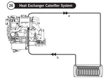
All Beta engines can be fitted with the calorifier connections to allow the coolant from the closed circuit cooling system to circulate through a calorifier tank, which in turn heats up domestic water. Calorifier connections on this range of engine are shown.
