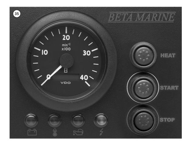
This panel controls the engine with three water resistant push buttons instead of a keyswitch, and is less prone to damage and corrosion from sea water spray.
