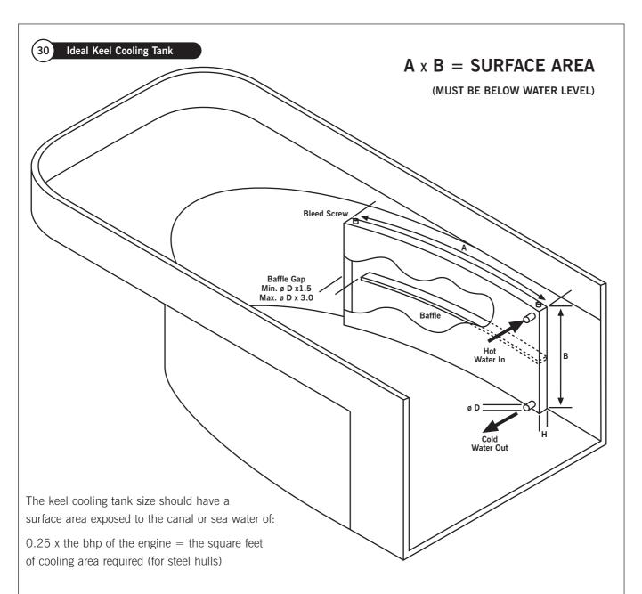
**NOTE:** If you boat has a hydraulic drive, you will need to increase the surface area by approximately 30% percent. Keel cooling pipes under the hull of yachts or work boats, that achieve the same surface area can also be used. If you have any questions about keel cooling please refer to our design guidelines detailed on our website, or ask us.
