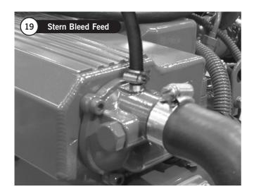
If your installation requires a water 'bleed' for stern gear lubrication of the cutlass bearing it can be taken from the engine as it leaves the heat exchanger.
