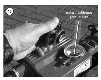
d) Fill header tank to the top of the filler neck and replace cap. Press down firmly on filler cap and hand tighten in a clockwise direction.
