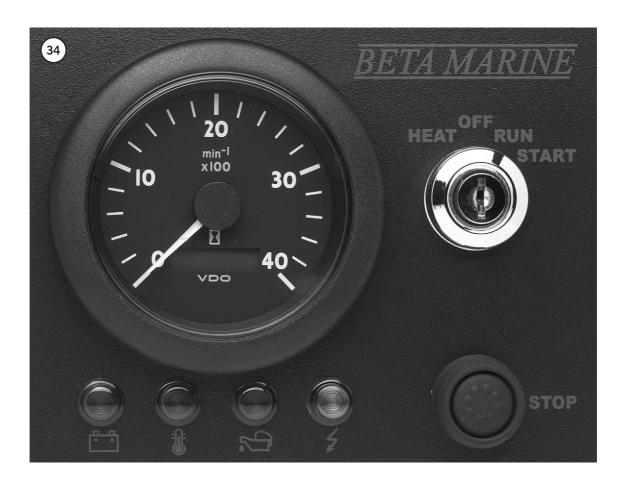
To operate the engine: with the engine out of gear, set speed control lever to 1/3 throttle.
