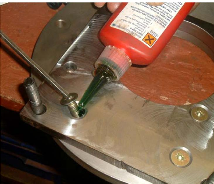
Bolt volvo adapter to super 5 adapter using M8 counter sunk screws provided with thread lock. (This may have already been finished for you).
