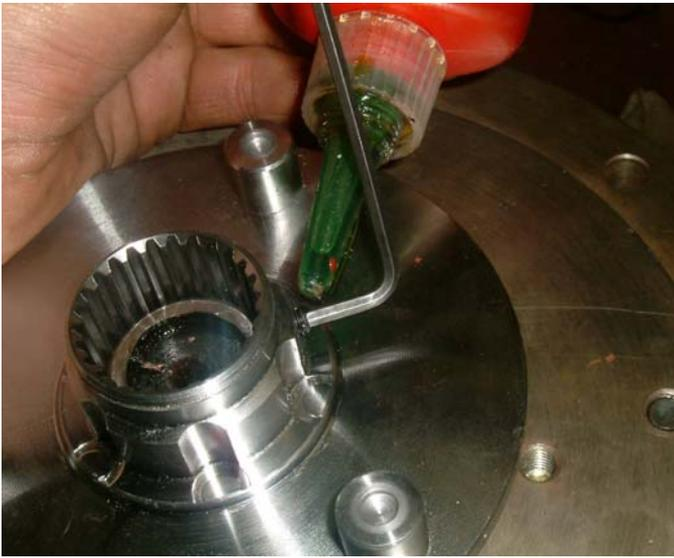
Once plate is in position lock grub screw onto shaft using small amount of thread lock.
