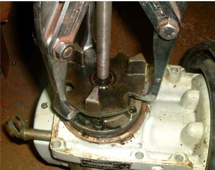
Remove the drive from the volvo leg as shown.
