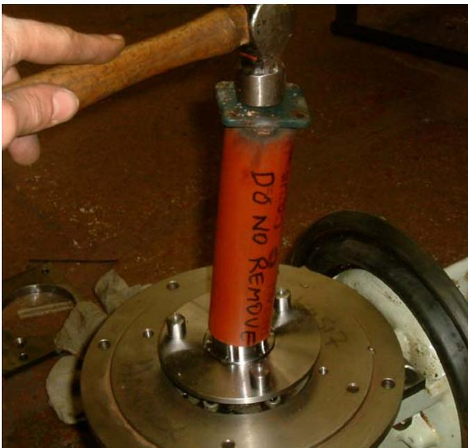
Align spline and knock driving plate onto shaft of sail drive. Fit until the plate is 23mm from point A to point B.
