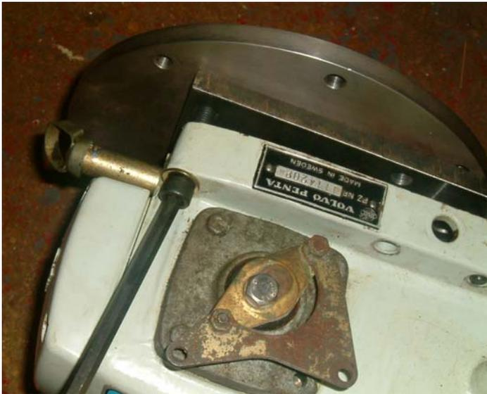
Bolt adapters the volvo sail drive using M10 cap heads and M10 nylock nuts provided.
